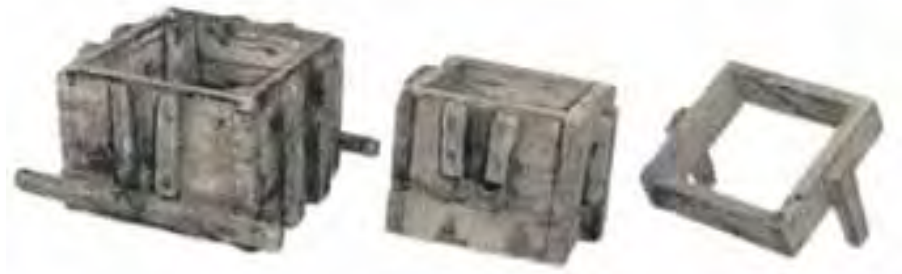
Wooden moulds, as used in casting at most iron works in the first half of the 19th century.
